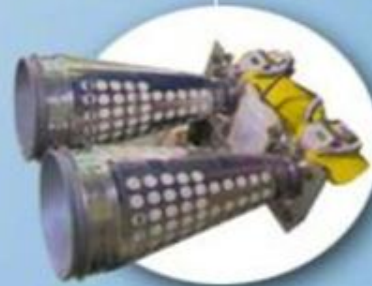
Re-arranged attitude control thrusters, DPO
