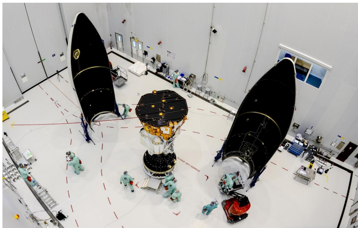
LISA Pathfinder fairing encapsulation in Kourou space-port, French Guyana. The LPF spacecraft seen from above while placed vertically with the fairing sides ready to be closed. (ESA)
