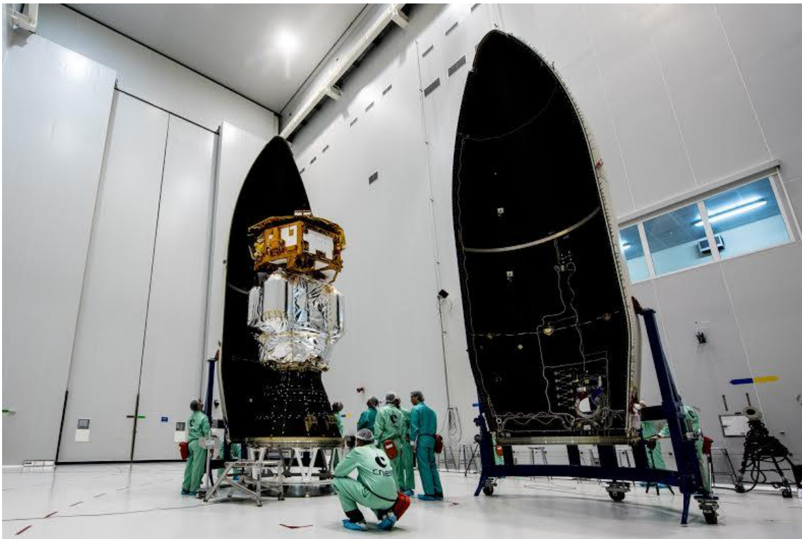
LISA Pathfinder fairing encapsulation in Kourou space-port, French Guyana. (ESA)
